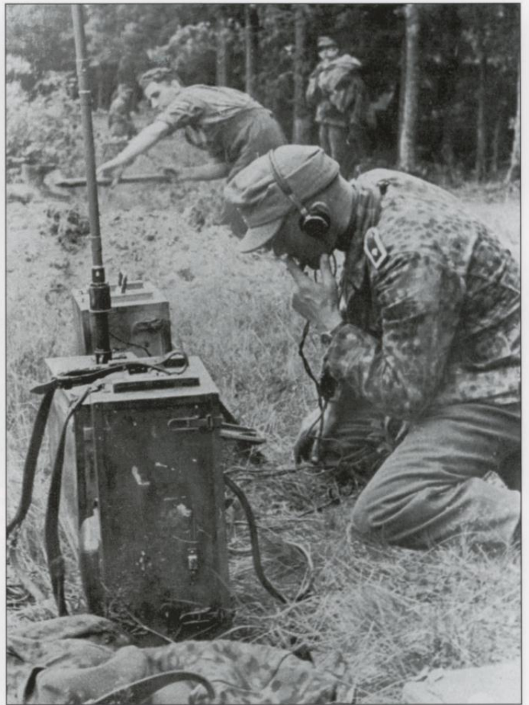
SS men dig in after taking up a position as part of an encircling cordon at the outskirts of a forest. Dressed in a camouflaged smock, the radio operator in the foreground sets up his equipment: a transmitter (with the antenna) and a receiver, a Totn. Fu. D (Tornister Funk D). Because of their size they had to be carried on the backs of two men.
