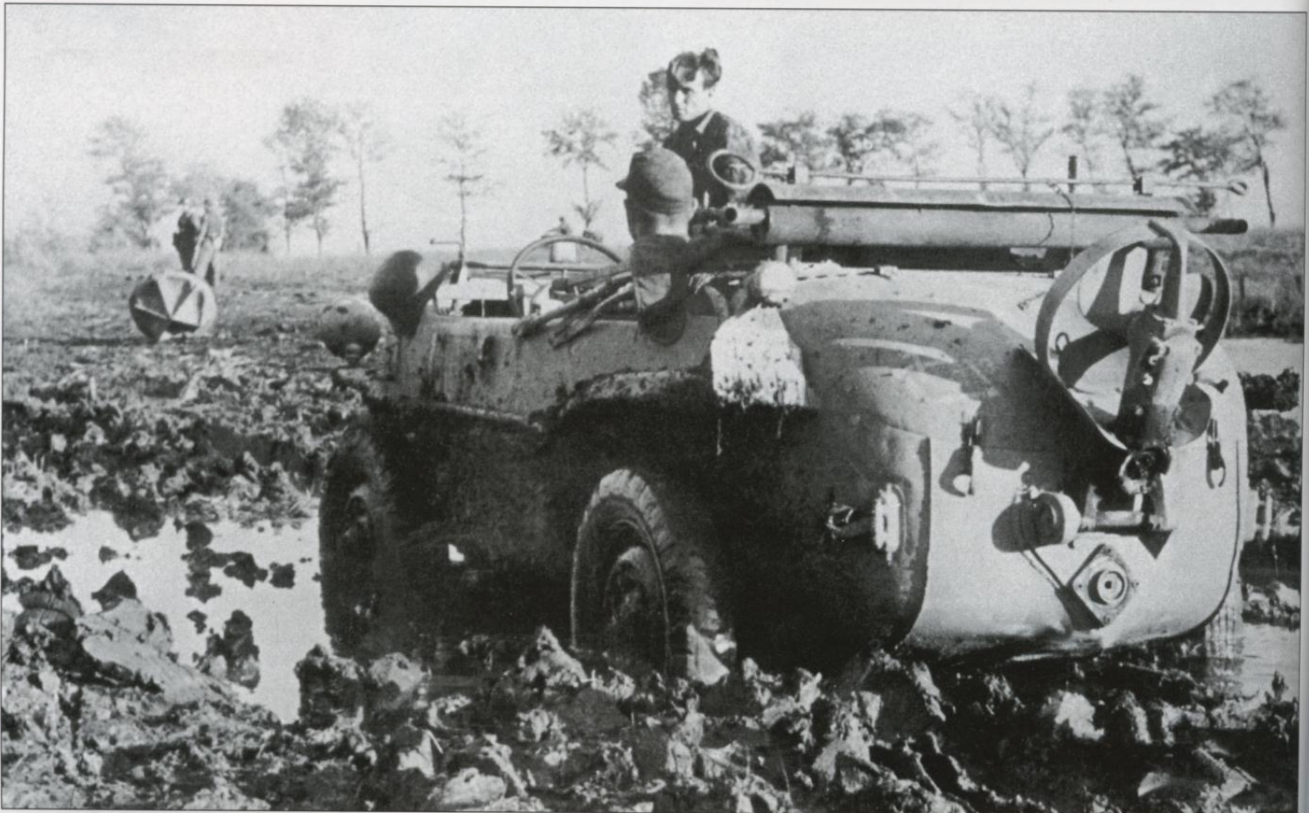
An SS Schwimmwagen slowly advances through the mire in a muddy stretch of land in Russia. If the terrain were any wetter, the driver would be compelled to lower the propeller at the rear of the vehicle to boost his speed. Note the markings that are visible just to the left of the propeller.
